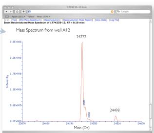
Color-coded sample plate view from 96-well oligonucleotide MS analysis. The deconvoluted mass spectrum from the green sample well A12 indicates the desired product was found as the major component. The mass spectrum from well C3 contained a major impurity, as indicated by the yellow color code.
