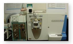
Novatia uses ion trap mass spectrometers, including the latest high-performance linear ion trap and orbitrap high-resolution mass spectrometers in our oligo MS services.
