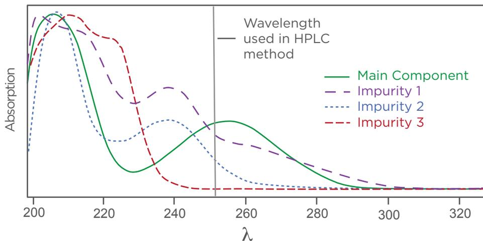
**FIGURE 1:** Varied UV-Vis absorbances of several species in a sample. Note that at the wavelength of interest, 254 nm, the Main Component shows the highest UV absorption while Impurity 3 shows little to no absorption.
