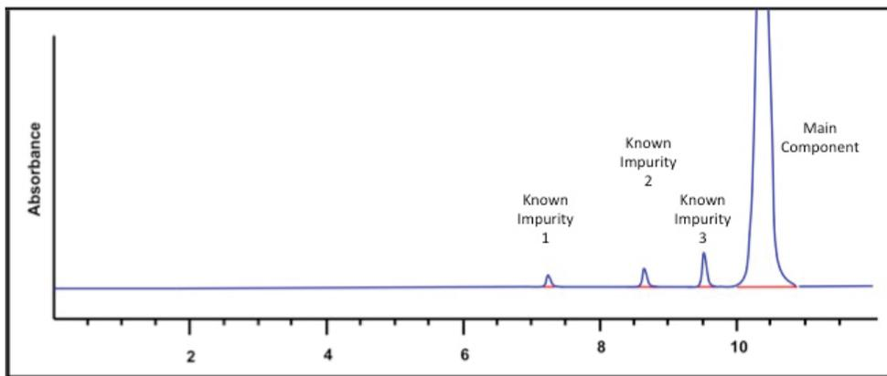
**FIGURE 4:** LC/UV chromatogram of sample containing unknown amounts of known impurities (top) and example conversion of area percent into Weight % using Relative Response Factors (bottom)
