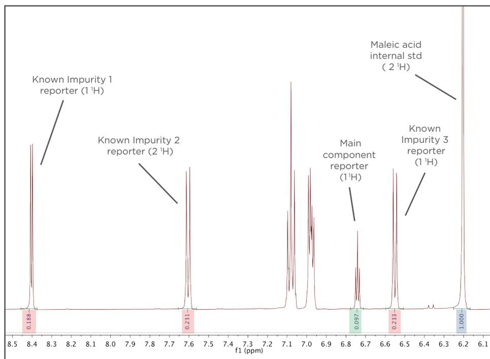
**FIGURE 2:** qNMR spectrum of an example impurity calibration standard containing unique reporter peaks of three impurities, a main component of interest, and maleic acid as the internal reference standard
